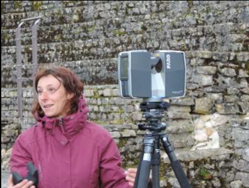
Terrestrial laser scanning: capturing 3D point clouds
