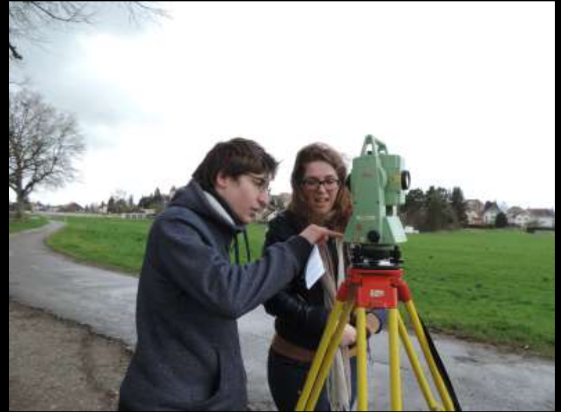
Total station: surveying of Ground Control Points
